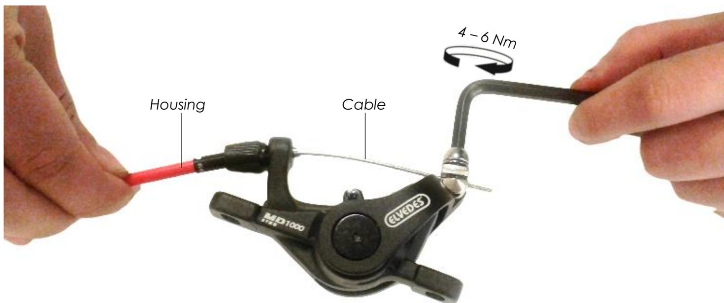
**A. Pull cable and tighten**
